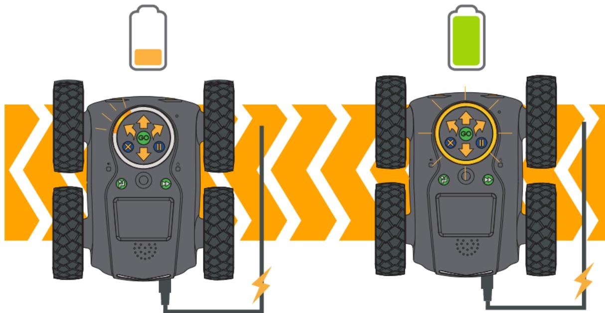
Battery: 3.7V, 850mAh Lithium polymer (Non replaceable)
